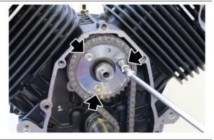
Remove the fixing screw with relative washer for the oil pump gear.
