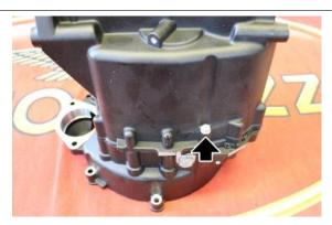
Insert the 12 fixing screws of the gearbox, engine side and then tighten them to the prescribed torque, including the screw opposite the cardan side previously tightened manually.
