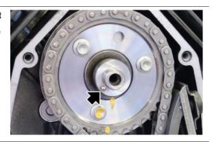
Insert the screw complete with washer to fasten the tone wheel and tighten it to the prescribed torque.
