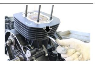
Slide off the cylinder from the stud bolts.
