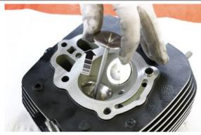
Remove the gasket of the valve guide
