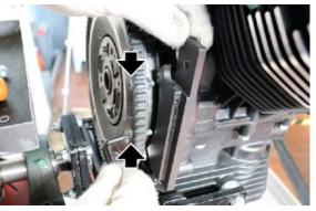
Using one of the fixing screws of the gearbox assembly, secure the specific tool.
