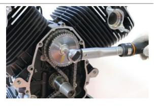
• Turn the crankshaft manually checking that there is no jamming. If jamming does occur, repeat the timing operation
