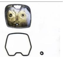
Check that the mating faces that contact the heads are not damaged or blistered
