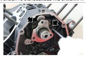
Remove the camshaft extracting it from the crankcase.
