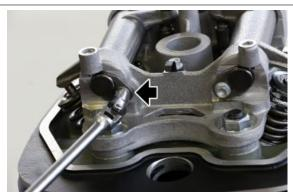
• Remove the rocker pin retainer fork
