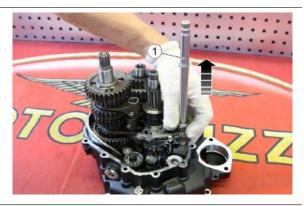
Remove the spring from the index lever
