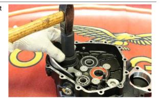
After installing the bearings on the gearbox crankcasings, position the bulkheads and the safety washers/plates, and tightening them with the appropriate screws to the prescribed torque.
