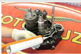
Position the gearbox cover and manually tighten the gearbox fixing screw on the cardan side.
