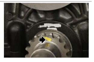
Having positioned the blow-by cap, fit the timing chain together with timing system gear and oil pump gear.
