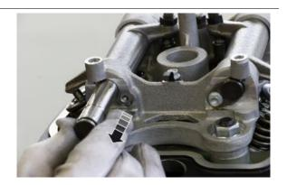
Remove the rocker, being careful to recover the Belleville spring
