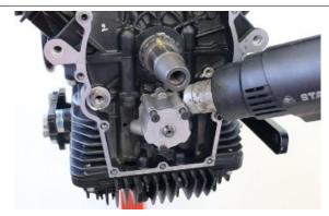
Remove the three fixing screws of the oil pump.
