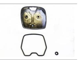
Place the head cover together with the gaskets on the seats of the fixing screws
