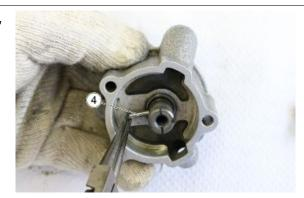
Insert the internal rotor (5) paying attention that the pin enters the machining seat.
