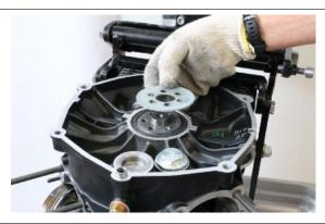
Insert the complete clutch lock.
