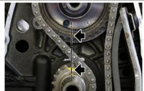
Using a thin tool, refine the alignment of the oil pump pin with the milling on the gear of the pump itself.
