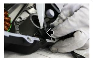
Check that plentiful threebond leaks out and covers all space between the seat on the cover and the cable grommet. Apply another layer of threebond over the cable grommet.
