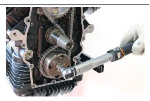
Position the three fixing screws of the timing gear and tighten to the prescribed torque.
