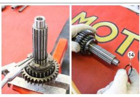
• Remove the gear of the 6th gear (15)
