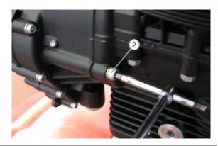
• Remove the complete gearbox screw
