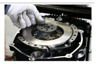
• Remove the clutch lock complete
