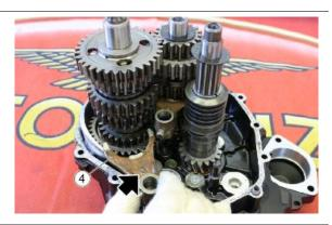
Remove the primary and secondary shaft, as well as the intermediate fok No. 2
