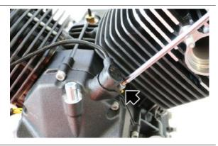
Remove the timing system cover sensor
