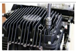
• Remove the engine oil filter
