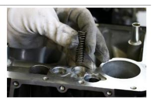
Remove the overpressure valve
