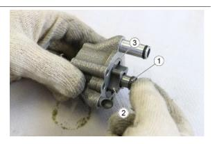
Working from the front of the oil pump, insert the internal rotor retaining pin
