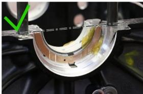
on the crankshaft and the assembly onto the engine crankcase making sure that the connecting rods locate correctly into their seats.
