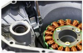
Removing the three stator fixing screws makes it possible to disconnect it
