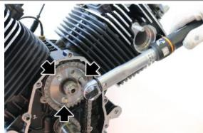
Position the tone wheel and after inserting the fixing screw with washer, tighten to the prescribed torque.
