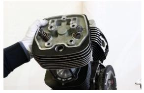
Remove the cylinder head gasket
