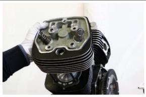
Place the three rubber O-Rings, particularly apply grease to the O-Ring that will be inserted in the stud bolt in order to avoid damaging it
