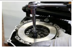
Remove the reinforcement flange of the clutch thrust plate
