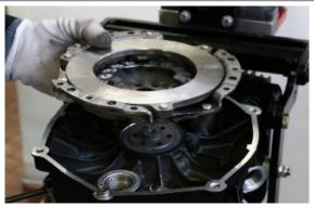
• Remove the spacer plate.
