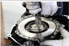
• Remove the thrust plate
