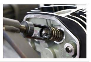
Close the tool to compress the spring and remove the two half-cones from the upper cap
