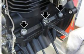
Undo and remove the four long nuts from the inside of the crankcase.
