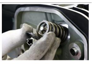
Remove the spring and replace it if it is out of the wear limit.
