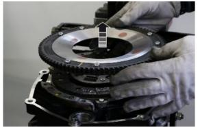
• Remove the clutch disc.
