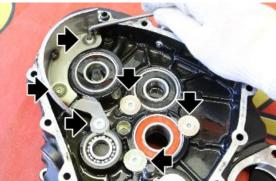
After inserting all the internal components, apply a layer of threebond on the junction surface of the two crankcasings.
