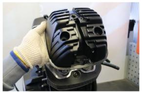
Place the cover fixing screws and tighten them to the prescribed torque
