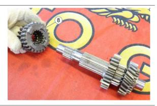
Using the appropriate jaws, lock the primary shaft in a vice and remove the circlip (9)
