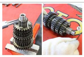
• Remove the gear of the 5th gear (6)
