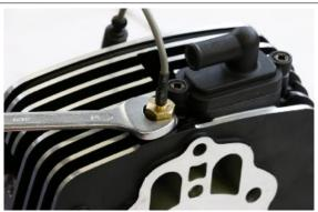
Undo and remove the secondary air valve cover
