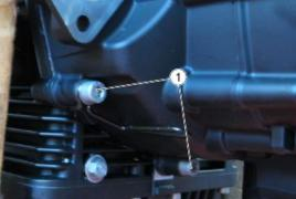
Remove the fixing screw (2) of the gearbox, placed from the engine crankcase side
