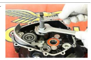
• Heat the primary shaft bearing area on the base of the gearbox crankcase and the secondary shaft area on the gearbox crankcase cover very well with a hair dryer. It will then be possible to remove the bearings by knocking the crankcasings on a surface. If necessary, use a dummy ball bearing extractor.
