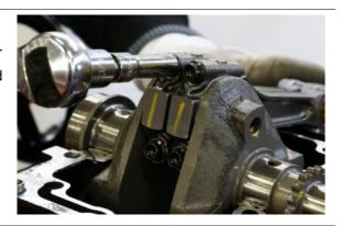
Remove the small ends from the connecting rods.
