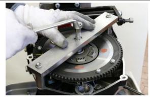
• Insert the six fastening screws at the recommended torque.
