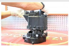
Having removed all internal components, to remove the bearings fitted in the gearbox crankcases, the safety washers/plate must be removed first.
