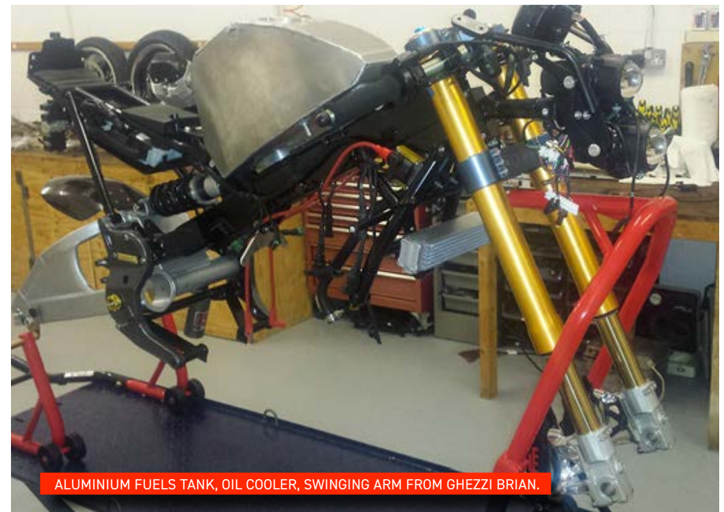
FORKS - ORIGINAL WHITE POWER USD FORKS WERE LONG. 800MM LONG. FORTUNATELY, OHLINS LISTED 800MM FG324'S FOR CUSTOM BIKE BUILDERS.
