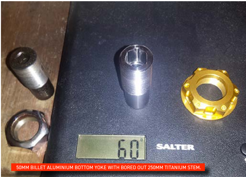
CHANGE TO TITANIUM SWINGING ARM PIVOT POINTS REPLACE ORIGINAL STEEL ITEMS, LOCKED IN PLACE WITH ALUMINIUM LOCK NUT.
